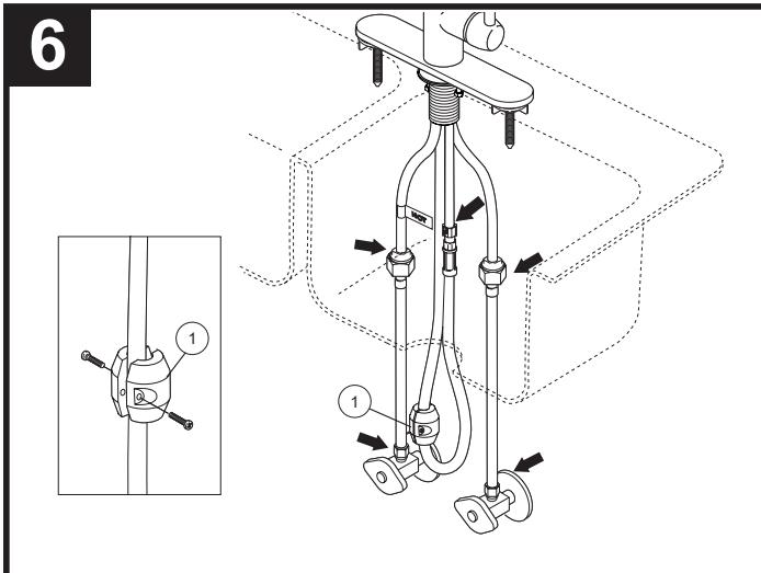
Attach the zinc weight (1) to the hose assembly in the approximate area shown. The weight should be on the upward swing of the hose, toward the spray head in order to provide proper pull to the hose. If further retraction is desired add a second weight. Make sure copper inlet tubes do not interfere with spray hose assembly. Hose assembly should pull freely through spout hub. Check all connections at arrows for leaks.
