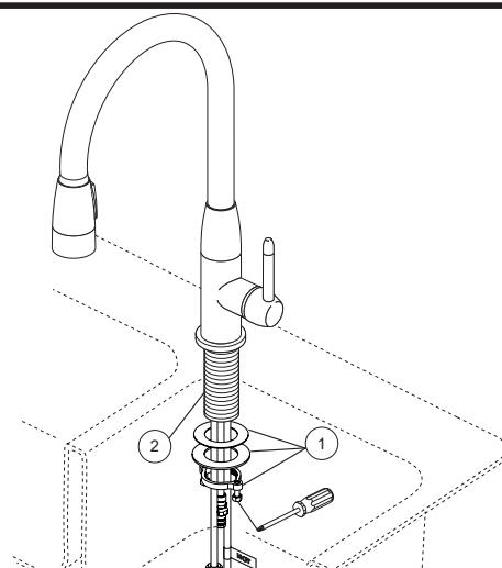
Make sure escutcheon is centered under faucet. Secure faucet by installing gasket, washer and nut (1) onto mounting shank (2). Tighten securely with phillips screwdriver.
