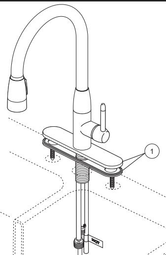
**Shut off water supplies.** Remove old faucet. Slide escutcheon and gasket (1) up over hose and tubes and underneath the faucet. Make sure the gasket is properly seated under the escutcheon, and place the faucet over the mounting holes.
