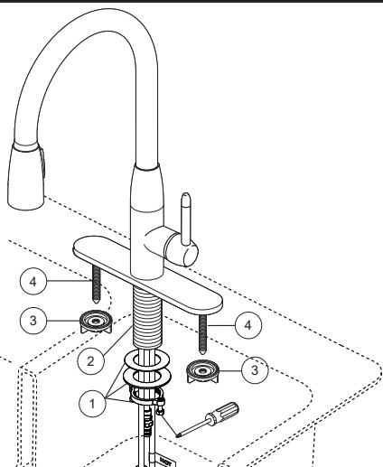
Make sure escutcheon is centered under faucet and parallel to the back splash. Secure faucet by installing gasket, washer and nut (1) onto mounting shank (2). Tighten securely with phillips screwdriver. Install locknuts (3) onto studs (4) and tighten securely by hand.
