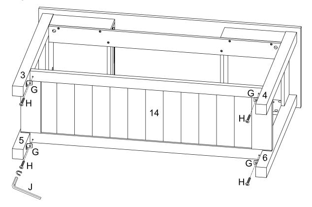
Use wrench (J) to secure shelf (14) to legs (3,4,5,6) with bolt (H) through L shape bracket (G).
