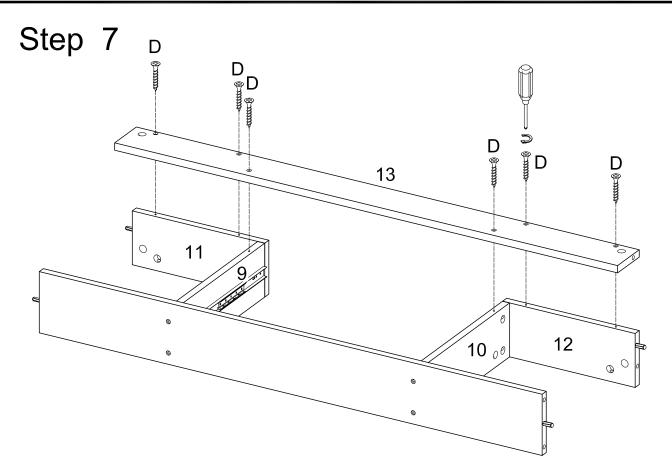
Secure bottom support bar (13) to middle side panel (9,10) and drawer front panel (11,12) with screw (D).
