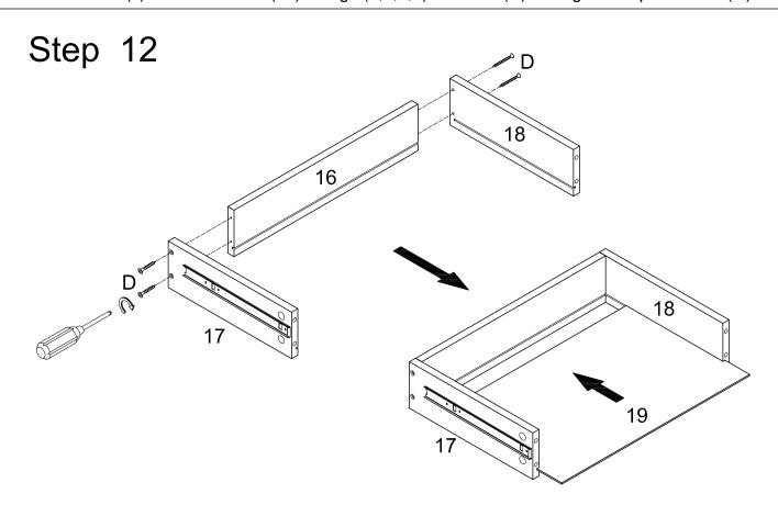
Secure drawer side panel (17,18) to drawer back panel (16) with screw (D). Insert drawer bottom panel (19) through side panel (17,18).
