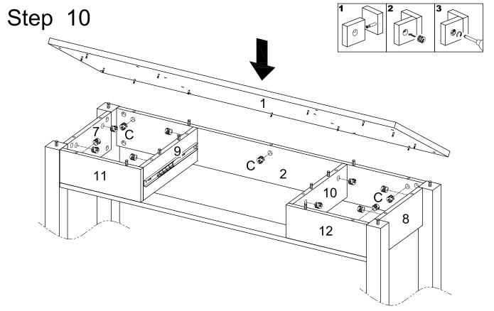
Insert top panel (1) into drawer front panel (11,12), side panel (7,8), middle side panel (9,10), and back panel (2), then insert and secure cam lock (C) to drawer front panel (11,12), side panel (7,8), middle side panel (9,10), and back panel (2) to lock it.
