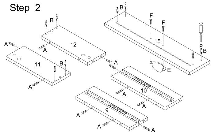
Insert wooden dowel (A) into front panel (11,12) and middle side panel (9,10). Secure cam bolt (B) to front panel (11,12) and drawer front panel (15). Attach handle (E) to drawer front panel (15) with bolt (F).
