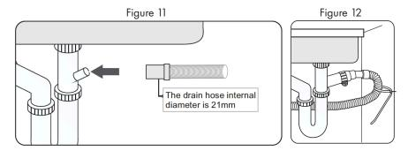
Figure 12: Secure the drain hose to the sink wall using cable ties or other fastening materials. Otherwise, the drain hose may bend at the end causing a drainage problem or excessive supply of water.
