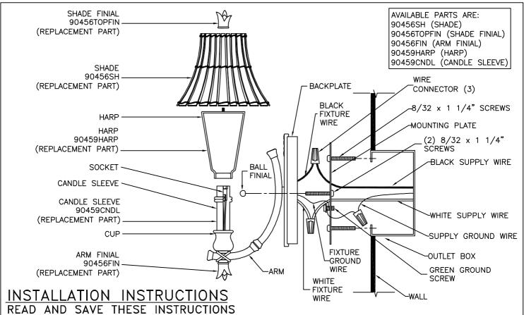
CAUTION: TO AVOID POSSIBLE ELECTRIC SHOCK, MAKE SURE THE ELECTRICITY IS SHUT OFF AT THE MAIN PANEL. IF YOU ARE REPLACING AN EXISTING FIXTURE, FIRST TURN THE FIXTURE OFF. NEXT, TURN THE WALL SWITCH OFF. FINALLY, GO TO THE MAIN FUSE OR BREAKER BOX IN YOUR HOME. TURN THE FUSE OR BREAKER TO THE OFF POSITION. SOME TYPES OF FUSES MUST BE UNSCREWED TO SHUT OFF THE POWER.
