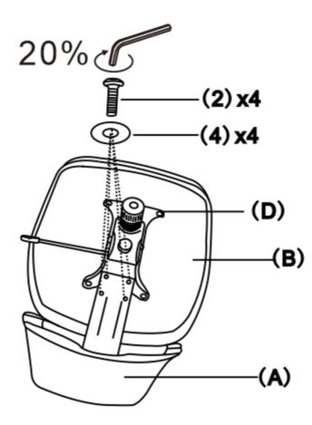
Attach the metal plate on Back (A) to the Mechanism (D) with four Long Bolts (2) and four Washers (4). Use Allen Key (6) to tighten approximately 20%.
