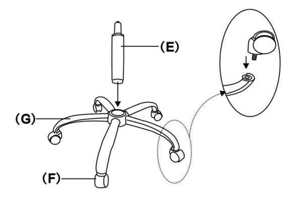
Place the Base (G) upside down on a flat smooth surface. Attach the Casters (F) to the Base (G). Attach Gas Lift (E) to the Base (G).
