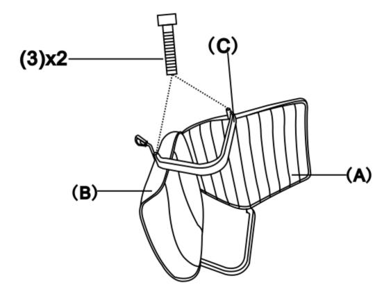
Attach the Arms (C) to the Back (A) and Seat (B) using two Flat Head Bolts (2) on each Arm (C). Use Allen Key (7) to tighten.
