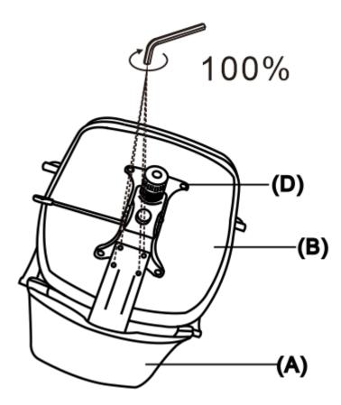
Place the Seat (B) on its back on a flat smooth surface. Use Allen Key (6) to fully tighten.
