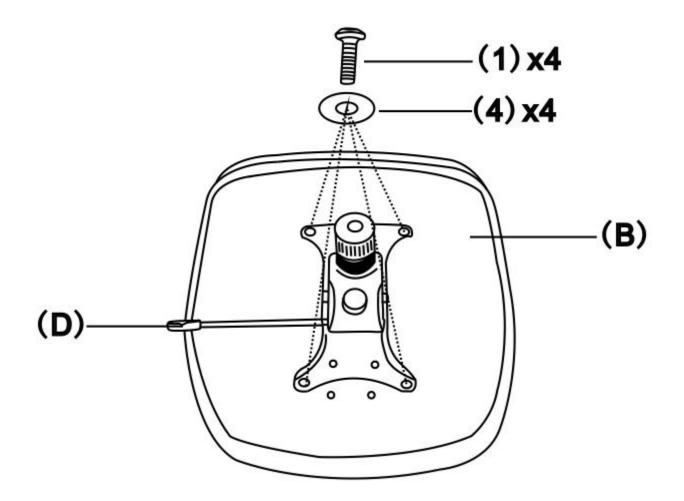
Place the Seat (B) on its back on a flat smooth surface. Attach the Mechanism (D) to the bottom of the Seat (B) with four Short Bolts (1) and four Washers (4). Use Allen Key (6) to tighten.
