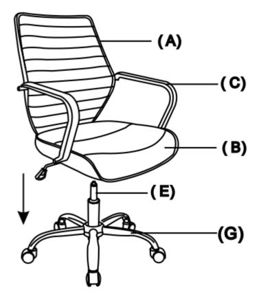
Place the Seat (B) right side up the Gas Lift (E).
