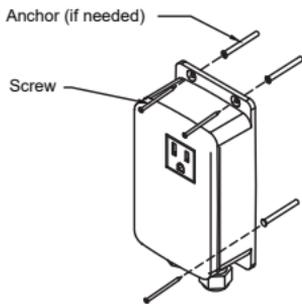
Mount the power module to the cabinet wall atleast three feet within an electrical outlet and the disposer.
