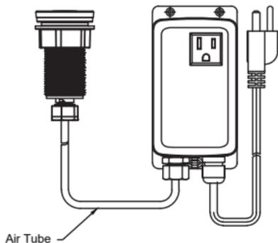
Attach air tubing between the push button and power module.
