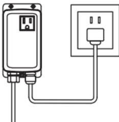
Plug the power module into a dedicated, grounded 120V AC outlet which is continuously energized.
