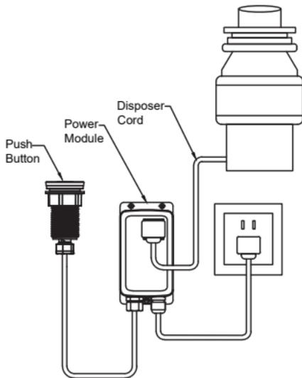
Plug the disposer cord in the power module.
