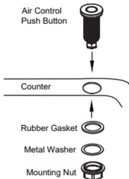
Mount the push button directly through a standard sink hole or drill a minimum 1 1/4" hole.
