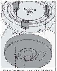
Align the the screw holes in the upper switch housing posts with the holes in the lower switch housing. Raise the switch housing to the upper switchhousing
