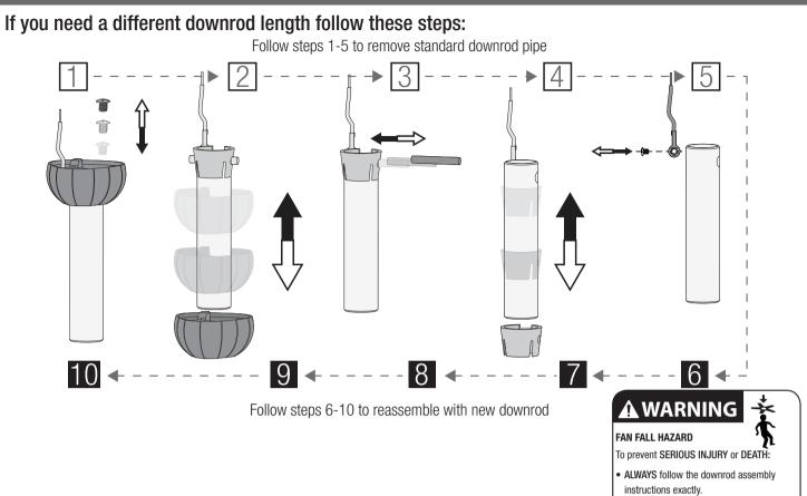
• VERIFY the downrod is assembled correctly by firmly pulling on the hanger ball.
