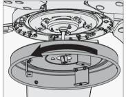
Feed the 9-pin plug connector coming from the bottom of the motor housing through the center hole in the light kit assembly. Align the keyhole slots in the top of the light kit assembly with the partially installed screws. Wrap the keyhole slots around the screws and twist counterclockwise.
