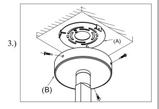
Step 3: Attach the body (B) to the mounting bracket (A) using three screws provided.
