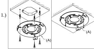
Step 1: Remove mounting bracket (A) from fixture and install to the ceiling, then install to electrical box.
