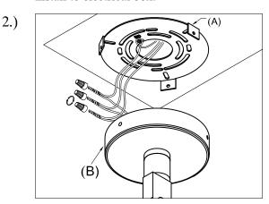
Step 2: Wire fixture to wire in outlet box. Copper wire is for ground
