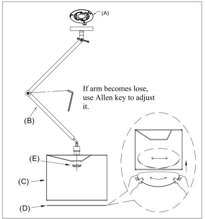
Step 4: Remove the socket ring (E) from fixture (B). Attach shade (C) and secure using socket ring (E). Insert acrylic diffuser (D) through the bottom of the shade.
