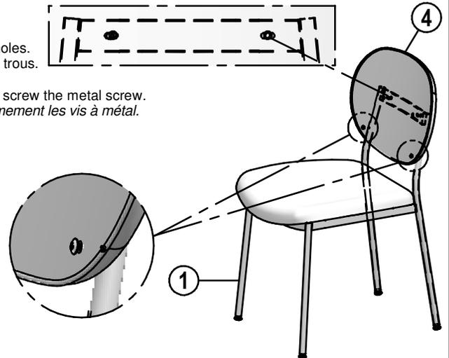
**7** 7.1 Align holes and screw lightly (bolts from step 1.1).
