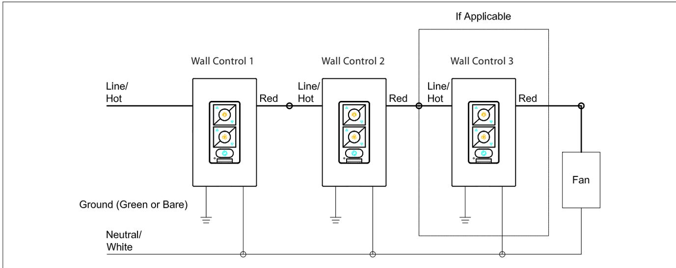
1. Install the wall control using the wiring diagram above.
