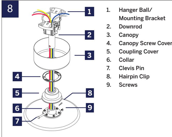
(painted side face down), and canopy (opened side up) onto the downrod. Coupling cover goes all the way to the bottom.
