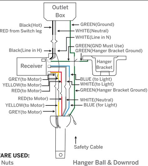
1. Connect the hanger ball/downrod assembly ground wire, mounting bracket ground wire and receiver ground wire to the ground wire in outlet box. Make sure all connections are made correctly or you will permanently damage the receiver. You may also refer to the labels on the receiver wires for direction on how to make proper connections. Use **D** Hardware.
