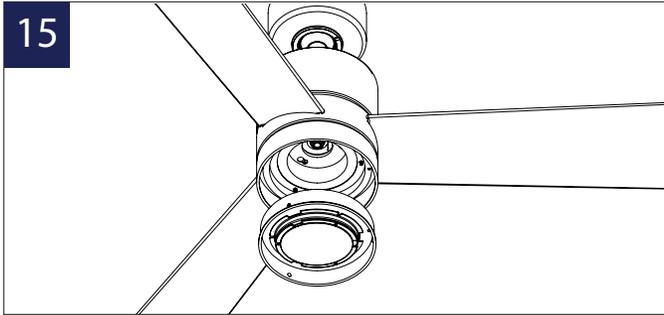
1. Remove 1 screw from the adapter plate for future use and loosen the two others from the outer perimeter of the adapter plate and keep for future use.
