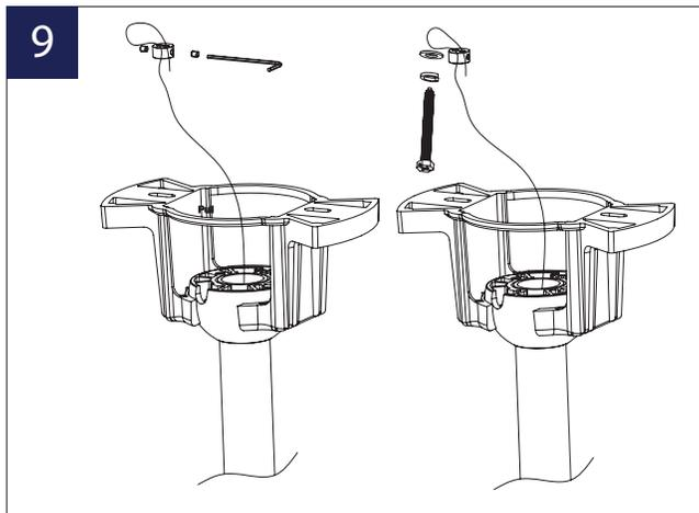
Make sure you have the correct downrod size prior to cutting said lead wire. Make sure the electrical supply wires, including the hanger bracket grounding wire and safety cable are pulled through the downrod, between the hanger bracket and the outlet box so that electrical connections can be made later.
