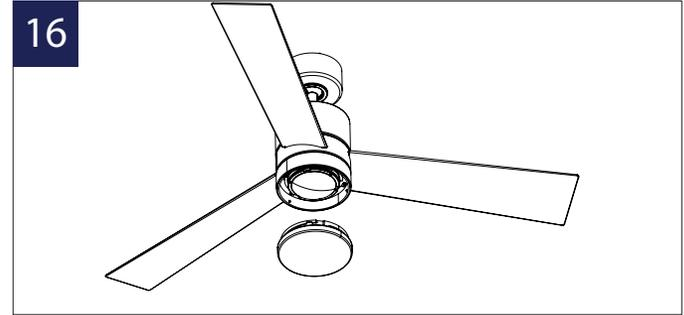
3. Tuck connections neatly into adapter plate. Place the luminaire module/plate and twist into key lock position. Tighten the two loosened screws and screw in the previously removed screw against the adapter plate. Raise glass shade up against the luminaire module, and secure it to fan by turning glass clockwise until snug.
