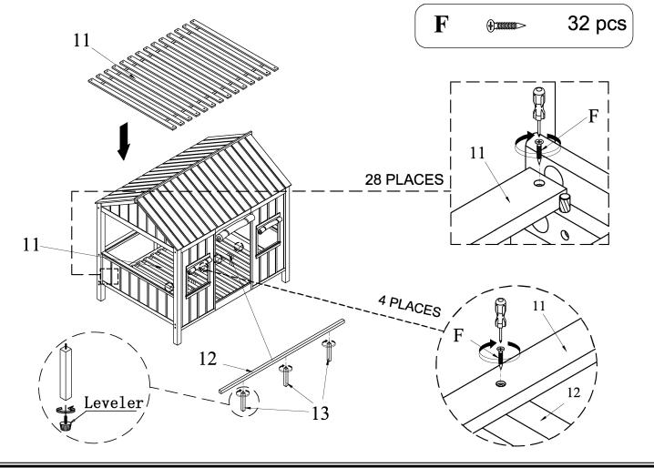
**STEP 8:** Front Support rail & Ladder Rail Assembly
