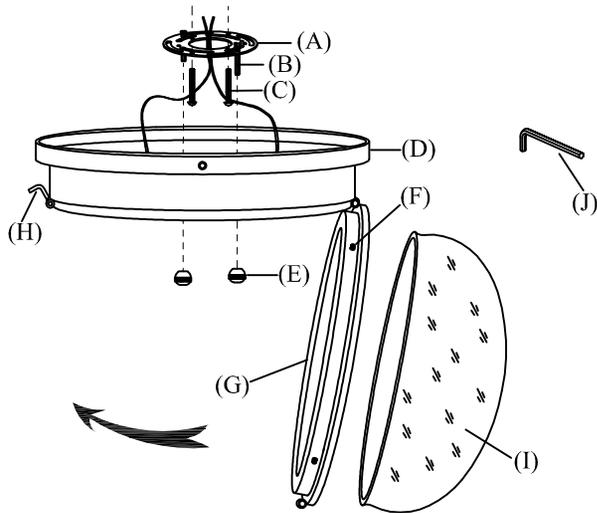
1. Remove back plate (A) with mounting plate (B) from fixture base (F) by unscrewing base screws (G).
