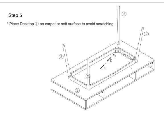
1.Attach legs  ${\bf \$}$  to underside of Desktop  ${\bf \^{1}}$  using bolts and allen wrench.
