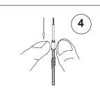
**4** Grasping the collar, slide braided outer wire back to expose inner wire. Trim 1/8" of insulation from the inner wire with wire stripper.
