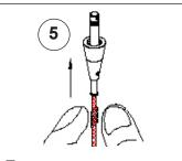
**5** Feed inner wire into quick connect adapter until it reaches top set screw. Feed braided outer wire and brass collar into quick connect.
