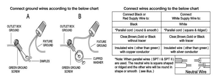
Twist wires together with plastic wire connectors until tightly joined, and wrap each connector with approved electrical tape. Be sure that no wire strands are exposed and then carefully tuck all wires into the outlet box.
