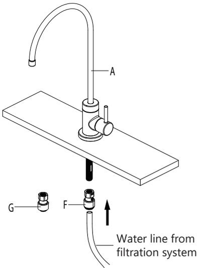
Thread the quick connect adaptor (F or G) onto the end of the faucet assembly (A) stud, and tighten securely using a wrench. Connect the water line from the filtration system by pushing the line into the connector (F or G). Pull down on the line slightly to ensure the quick connect fitting has engaged.
