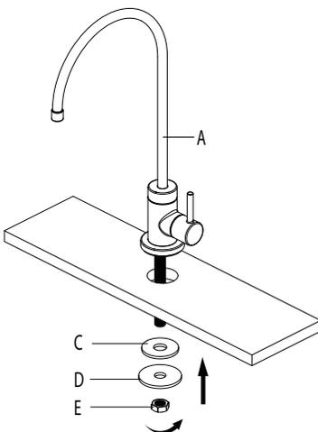
Place the faucet assembly (A) through the selected hole in the sink or countertop. On the underside of the sink or countertop, slide the rubber washer (C) and metal washer (D) onto the stud. Thread the mounting nut (E) onto the stud, and tighten securely using your wrench.
