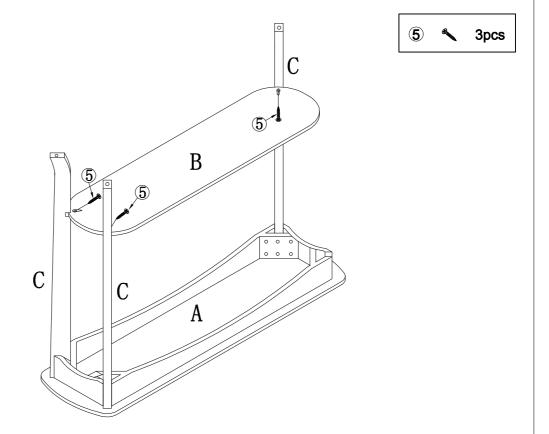
Insert Bottom Panel (B) into the grooves on Legs (C), then tighten Bottom Panel (B) to Legs (C) using Screws (5). NOTE: It is recommended that this step should be assembled by two persons.
