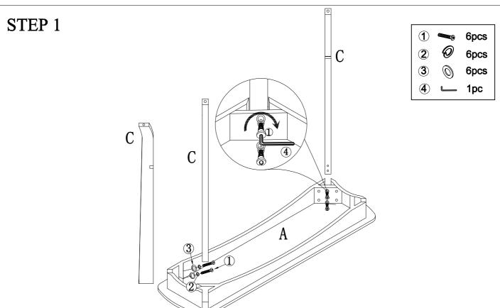
Assemble three Legs (C) to Top Panel (A) using Bolts (1), Spring Washers (2) and Flat Washers (3). Please do not tighten Bolts (1) until step 4.
