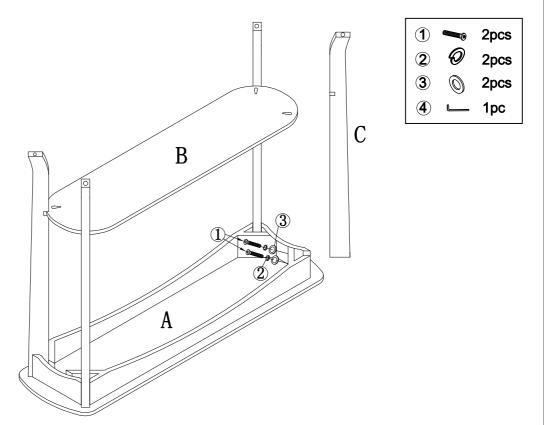
Assemble the 4th Leg (C) to Top Panel (A) using Bolts (1), Spring Washers (2) and Flat Washers (3) as above drawing shown. Please make sure that the Bottom Panel (B) is inserted into the grooves of the legs. Please do not tighten Bolts (1) until step 4.
