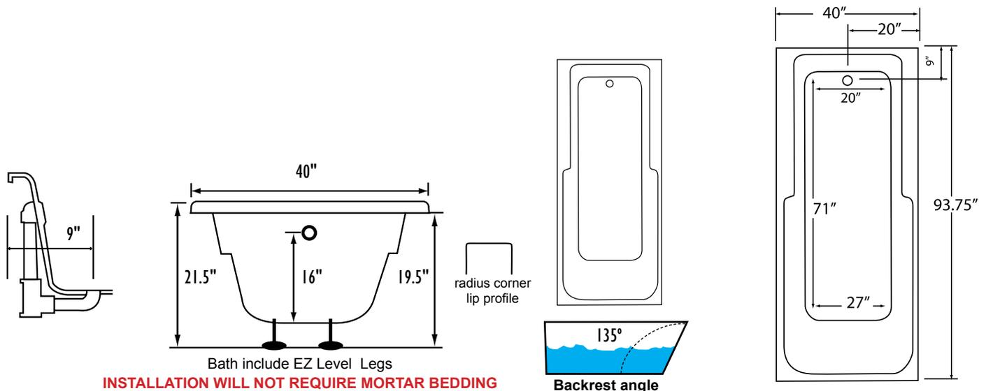
Some standard & most alternate pump locations may stickout past perimeter of the bath 1"-3". NOTE: Graphics may not be to scale. Specifications and features are subject to change without notice and are  $\pm .25"$ . All final measurements should be taken from tub on site. Access 18"x 18" or larger is required for each pump. Consult your contractor for installation requirements.
