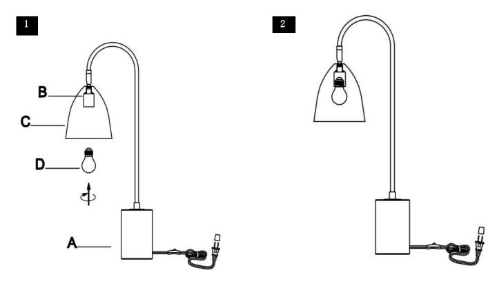
Step 1 Insert the bulb (D) into the socket (B).
