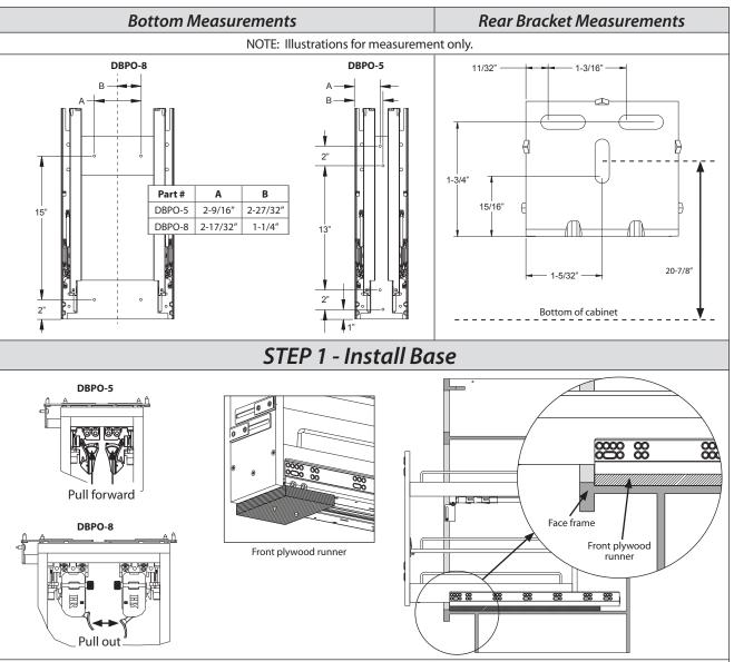
Remove the base from the unit by releasing the slide clips. In framed cabinets, center the unit in the opening making sure the front plywood runner is pulled tight against the back of the face frame. For frameless cabinets, place the unit within 1-1/2'' of the left of the cabinet and the front plywood runner needs to be set back 3/4''. Install with the four (4)  $#10 \times 3/4''$  Pan Head Wood Screws provided in the four pre-drilled holes in the runners.
