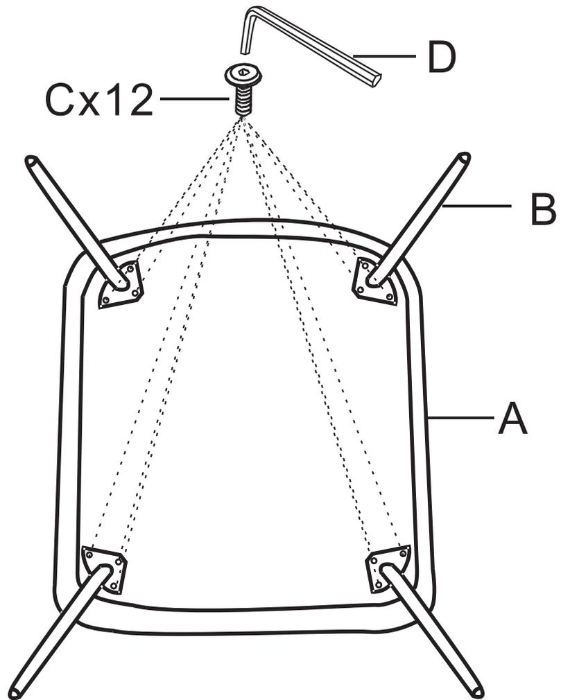
**STEP 2** :Use bolt C, allen key D to connect the metal leg B to bottom of the seat cushion A, make sure all holes align, fasten all bolts to secure.
