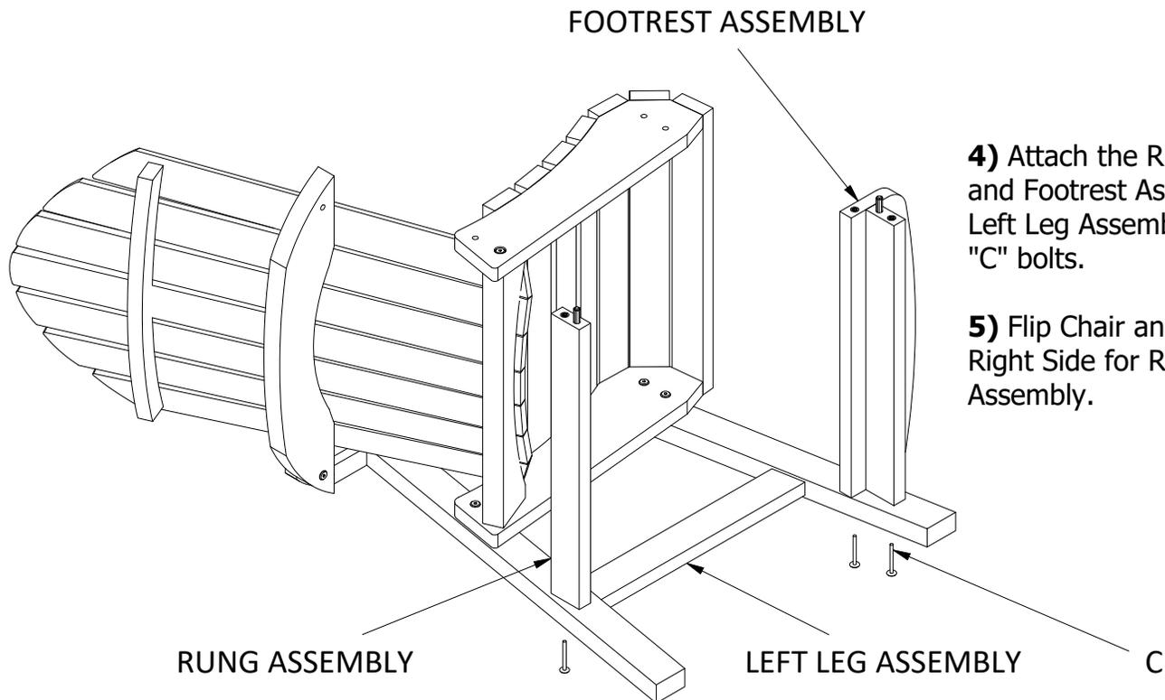
**4)** Attach the Rung Assembly and Footrest Assembly to the Left Leg Assembly using (3) "C" bolts.
