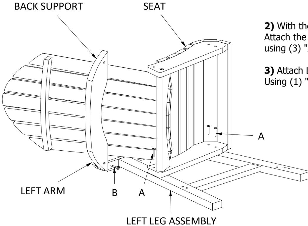
**2)** With the Chair Laying on its Left Side, Attach the Left Leg Assembly to the Seat using (3) "A" bolts.
