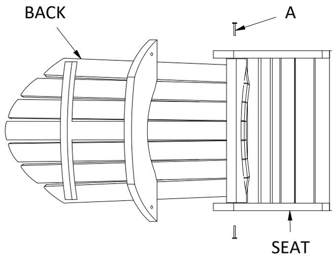
**1)** Insert (1) "A" Bolt into Lower Hole on Each Side to Attach Seat to Back. Make Sure the Back is Fully Upright. Make Bolts Snug, but Do Not Overtighten.
