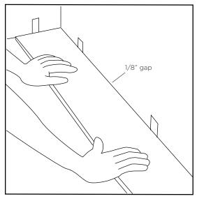
1.Lay a row of loose planks without securing them to each other first to derterimine if you need to adjust the length of the first plank to avoid a small piece of length of 12" on the opposite wall from where you start.
