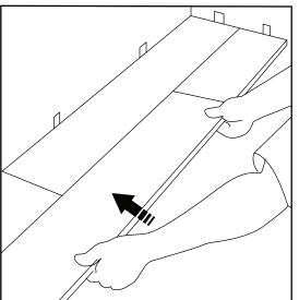
2.When installing, stagger the rows so that the short edge seams are not in a staright uniform ine. To start the second row with plank cut at about 2/3 length. Score the plank and snap. The next plank, interlock the short side first, leaving it slightly aways from the long side and then slide into the long side.
