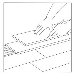
4.Continue this pattern for the remainder of the rows to be installed. Always place the cut end of the first plank against the wall. Fitting around irregular objects is no problem. Simply make a pattern out of heavy paper to fit around pipes or irregular objects. Place the pattern upon the plank and trace. Cut along trace lines using a utility knife, and lay plank. Be sure to leave a minimum of 1/8" expansion space around all fixed objects, floor vents and door frames.
