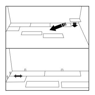
3.When cutting for length, be sure to always cut the short side of the plank with the groove edge. The remaining piece can then ne used on the opposite side of the room, at the end of that row of layout permits.Start the third row with the plank cut at 1/3 of a length. Again the remaining piece can be used at the opposite end of the row, if the layout of the room permits.
