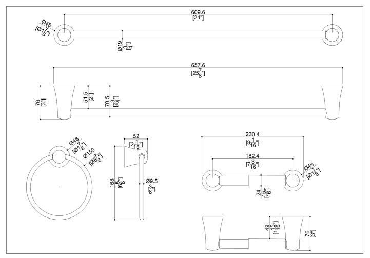
Column kit composed of column expandable roll paper holder, column towel bar and column towel holder, polished
