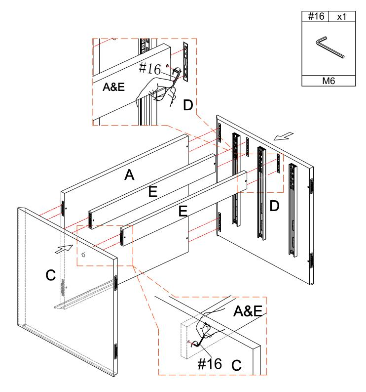
1. insert pre-assembled unit at step 1 to bottom panel(B),make sure all holes aligned and then tighten it with allen key #16 as picture show.
