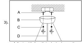
Adjust cable length to desired mounting Step.3: height, and tighten strain relief screws to secure. Install body (D) to bracket (A) and tighten finials (C) on the canopy (B) to secure.
