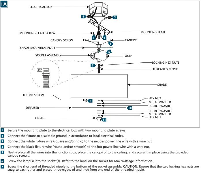
8 Align the shade to the shade mounting plate so the holes on the top of the shade line up with the holes in the shade mounting plate, then use the thumb screws to secure the shade to the plate.
