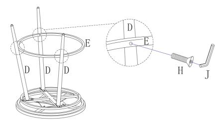
Attach Legs ( D ) to the Upper Ring ( A ) and Bottom Ring ( E ), using Bolt ( G ), Bolt (H) and Allen Key ( J ) to tighten.
