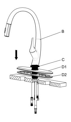
Insert the faucet assembly (B) through the hole in the deck plate assembly (D).
