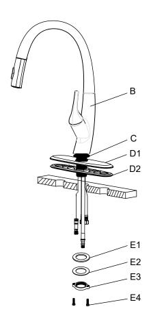
Insert faucet body (B) into hole on countertop or deck plate assembly (D) with base o-ring (C) attached. Attach mounting hardware (E).
