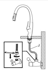
Thread hot & cold waterlines (J) onto angle stops. Tighten with adjustable wrench until snug. Turn on the angle stops and check for leaks.
