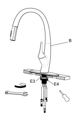
Adjust faucet body (B). Tighten mounting nut (E3) with wrench and mounting screws (E4) with Phillips head screwdriver.
