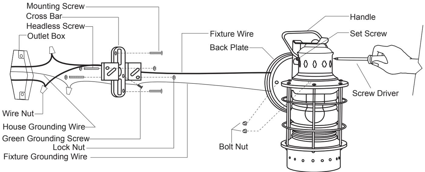
1. Thread two headless screws through the cross bar, then secure them with four lock nuts (two on each side of the cross bar). Adjust the length of the headless screws if necessary.
