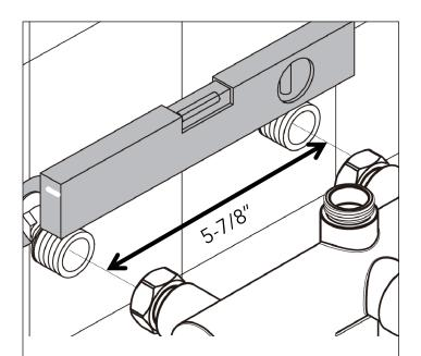
**3.** Adjust the adapters so they are level and exactly 5-7/8" apart on center.
