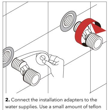
tape to ensure a watertight seal.
