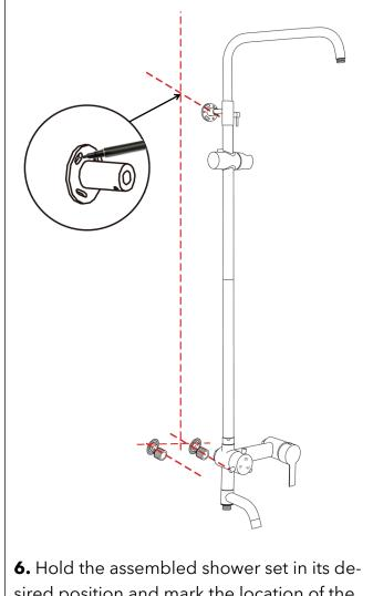
sired position and mark the location of the mounting bracket.
