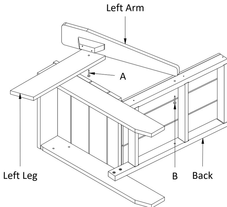
**3)** With the chair still on it's side, attach Left Arm to Back using one B bolt as shown. Attach Left Arm to Left Leg using one A bolt as shown.
