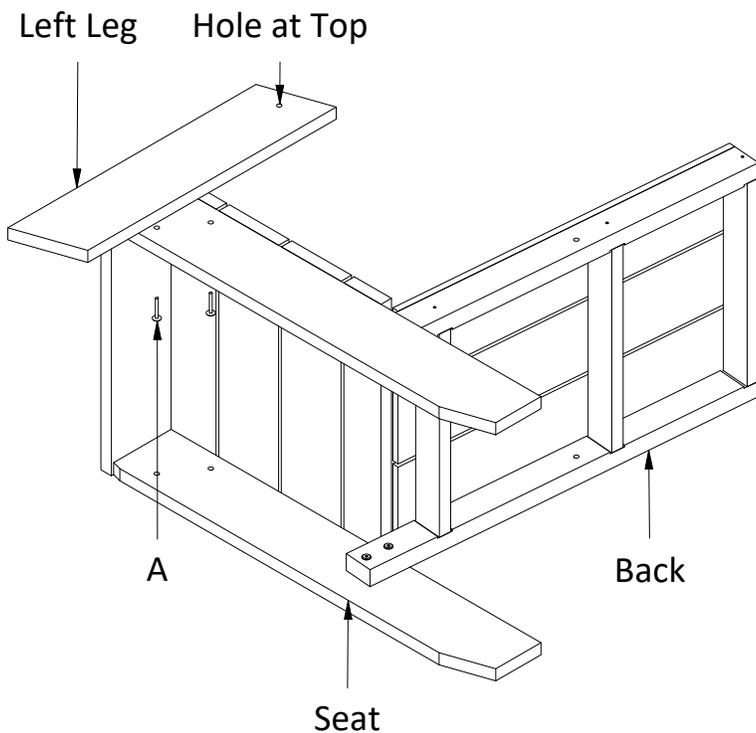
**2)** With the Back and Seat on their sides, attach Left Leg as shown to Seat using two A bolts.
