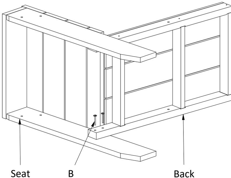
**1)** With the Back and Seat on their sides, attach one side of the Back to the Seat using two B bolts.
