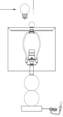
Step2 Insert the bulb(G) into the socket(C).
