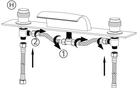
Secure water line connections to each corresponding faucet handle shank base.
