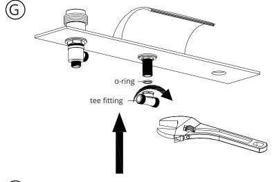
H. Attach the hot and cold supply lines to the Tee fitting at the faucet base.
