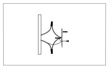
1.Remove mounting bracket from fixture and install to electrical box. Then wire fixture to wires in outlet box. Copper wire is for Ground.
