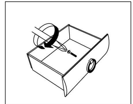
**NOTE :** MUST TIGHTEN SCREWS **PERIODICALLY** WITH USE SCREW WILL BECOME LOOSE CHECK TIGHTNESS OF ALL SCREW EVERY 6-8 WEEKS.
