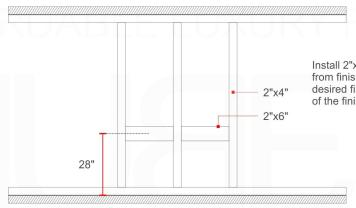
Install 2"x6" lumber between the wall studs. Suggested distance from finished floor will be 28" to the center from the floor if the desired finished height of the Vanity is 34" from the floor to the top of the finished countertop.
