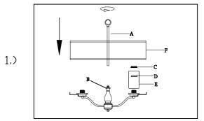
Step.1: Attach glass (E) to fixture using socket ring (C) and spacer (D) to secure. Add medium base bulbs. Attach shade (F) to fixme using screws. Run wire through stem (A), then carefully attach to fixture (B).
