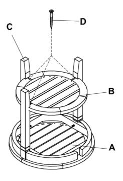
Attach the Tray (B) to the legs (C). Secure using 1 1/4" screws (D).
