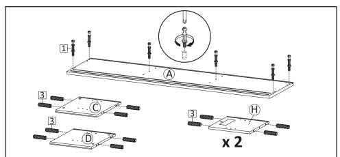
**STEP1**: Insert Cambolt (HW1) into Top Board (A). Insert Dowel (HW3) into Side Board Left (C), Side Board Right(D) and Center Board (H) as figure.
