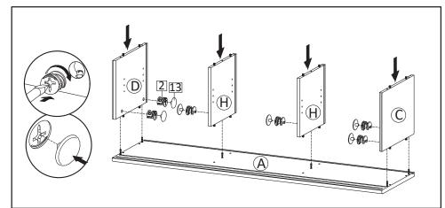
**STEP2**: Attach Side Boards (C&D) and Center Boards (H) into Top Board (A). Insert Camlock (HW2) then tighten using screwdriver. Put Screw Cap (HW13) over the camlock as picture.
