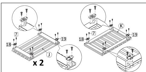
**STEP13**: Insert Sliding Top (HW18) and Sliding Bottom (HW19) using Screw M3.5x13mm (HW7) into Door 1 (J) and Door 2(K), tighten with a screwdriver position as shown in the figure.
