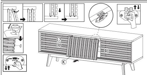
**Step15**: Install the doors 2 (K) and insert the Sliding Top (HW18) pin into the front groove line of the Top Board. Position the Sliding Bottom (HW19) into the sliding track of Bottom Board. Adjust gap of the door, by scroll the button on Sliding Roller (HW19). Follow the down and up direction. Slide both doors to right and left ensuring the door has been placed properly in the front sliding track.
