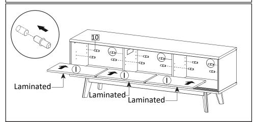
**STEP12**: After bringing the product upright, insert Shelf Pin (HW10) into the holes on Side board & Center board, on the desired level. Then place the Adjustable Shelf (I) by inserting the grooving on the shelf into the shelf pin.
