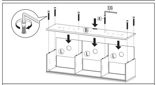
**STEP3**: Attach Back Board (L) and Insert Bottom Board (B), secure with Screw M7x50mm (HW4), tighten screws using Allen Key (HW16).
