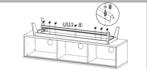
**STEP11**: Place Anti-Deflection Bar (HWUS11), secure with screw M6x12.5mm (HW8), tighten using screwdriver.
