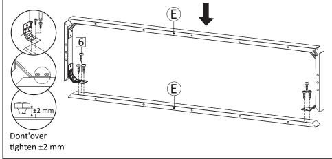
**STEP6**: Combine components from step 5 with remaining Bottom skirt 1 (E), using Screw M4x16mm (HW6). Do not overtight screw yet,leave around 2mm gap.
