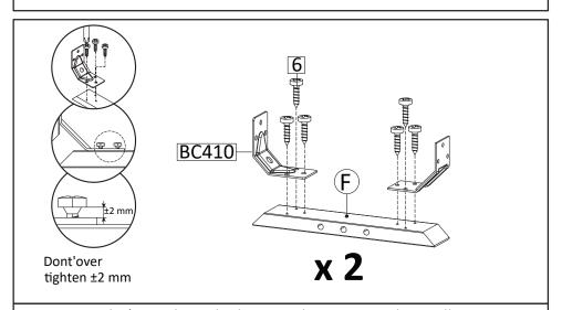
**STEP4**: Now let's combine the bottom skirt. Start with installing Corner Brace (HW BC410) into Bottom Skirt 2 (F) using Screw M4x16mm (HW6). Do not overtight screw yet, leave around 2mm gap.
