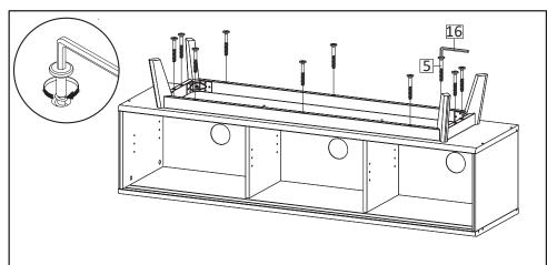
**STEP10**: Insert Screw M6.4x53mm (HW5) using Allen Key (HW16) into assembled bottom skirt.
