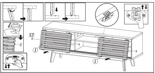
**Step14**: Install the doors 1 (J) and insert the Sliding Top (HW18) pin into the back groove line of the Top Board. Position the Sliding Bottom (HW19) into the sliding track of Bottom Board. Adjust gap of the door, by scroll the button on Sliding Roller (HW19). Follow the down and up direction. Slide both doors to right and left ensuring the door has been placed properly in the back sliding track.
