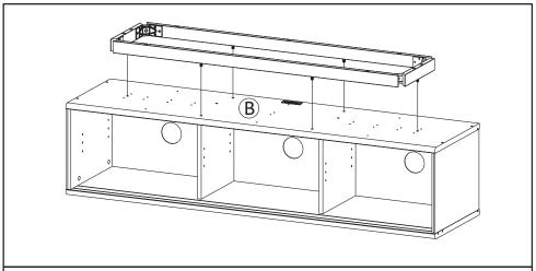
**STEP8**: Bring the assembled bottom skirt and insert into Bottom Board of the media stand.
