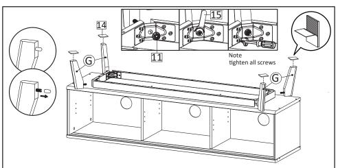
STEP9: First, let's fixing the leg by inserting leg to Corner Brace, Insert Flange Nut (HW11) first into the hanger bolt of leg, tighten all the Flange Nut using provided Wrench (HW15). Second, after ensuring that all legs has been tightened, continue with tighten all screws on the corner brace. Peel off paper from Floor Protector (HW14) and stick it onto the leg.
