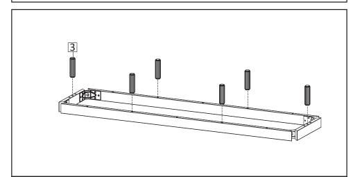
**STEP7**: Insert Dowel (HW3) into assembled Bottom skirt from previous step.
