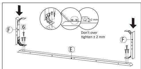
**STEP5**: Combine the Bottom Skirt 2 (F) from step 4 with Bottom skirt 1 (E),using Screw M4x16mm (HW6). Do not overtight screw yet, leave around 2mm gap.
