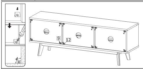
**STEP16**: Use Wedge (HW12), Screw M3.5x15.5mm (HW9) to tighten the back of media stand by using screwdriver. Please align the top board and bottom board in  $90^{\circ}$  position against the side board, before securing the wedges (HW12).
