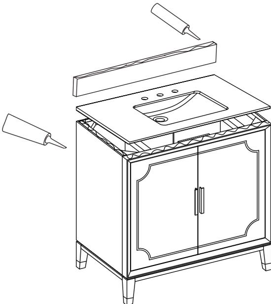
Apply bead of quality sealant evenly along the bottom of back splash and the top of the vanity.
