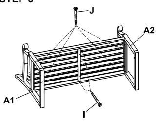
Secure the seat (C) using 1 1/2" screws (I) and 1" screws (J), as shown.
