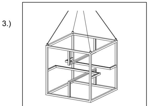
Step.3: Adjust wire length to desired mounting height, and tighten strain relief screws to secure.
