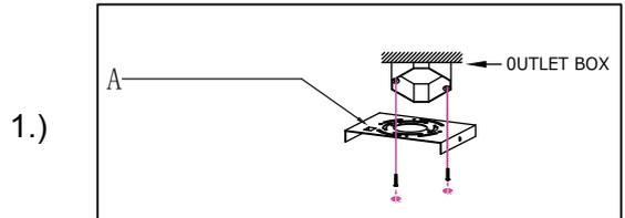
Step.1: Remove Mounting Bracket (A) from Canopy(C) to install to electrical box.
