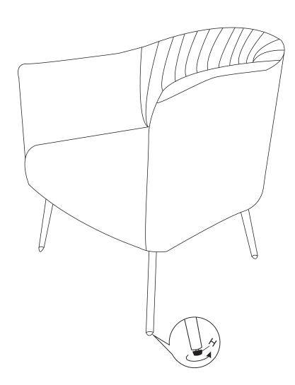
**STEP 2**: Use bolt C, allen key D to connect the metal leg B to bottom of the seat cushion A, make sure all holes algin, fasten all bolts to secure.
