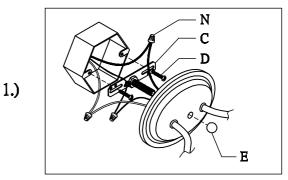
Step 1. Remove mounting bracket (C) from fixture and install to electrical box. Then wire fixture to wires in outlet box. Copper wire is for Ground.
