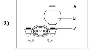
Step 2: Use the socket ring (A) to secure glass (B)on socket (F).
