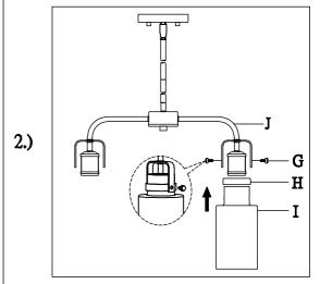
Step.2: Attach metal ring (H) and glass (I) to yoke and secure using set screws(G).
