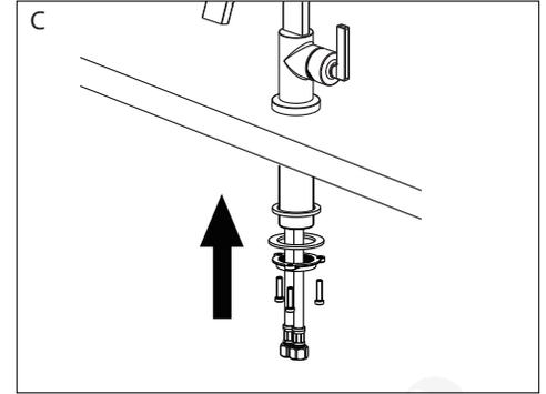
C. Under the sink, slide the washer and metal washer onto the faucet. Secure the faucet with the locking nut and screws to the countertop.
