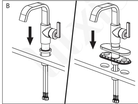
B. Use the flange for a single hole installation OR use the included deck plate to convert a 4 inch centerset hole pattern to a single hole pattern.
