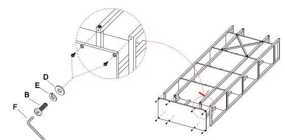
Do not tighten up all the bolts until each part is properly assembled.
