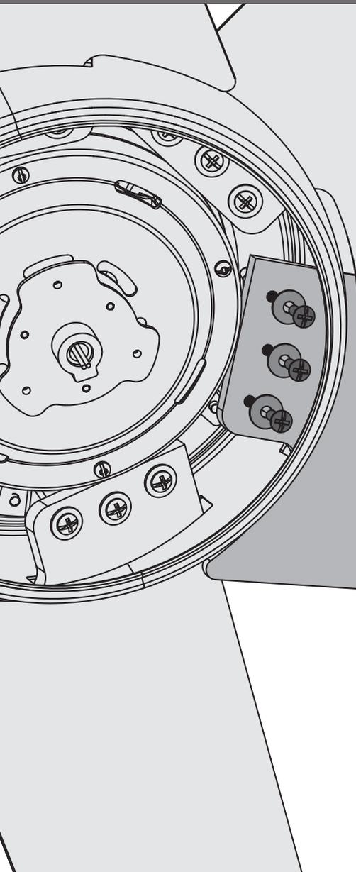
Attach each blade to a blade iron using three blade washers, found in the ■ hardware bag, and three blade assembly screws, found in the ▲ hardware bag.
