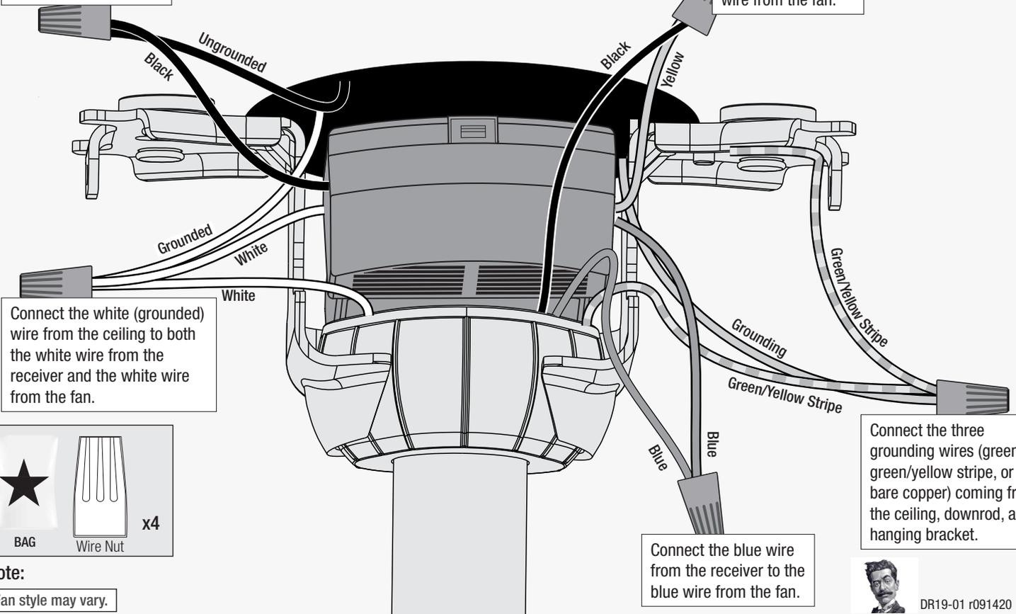
Connect the white (grounded) wire from the ceiling to both the white wire from the receiver and the white wire from the fan.
