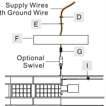
B. Optional Swivel: Install the swivel to the Shade (I) and then attach Nipple (G) and the Ceiling Canopy (F) to the Swivel using the Flat Washer (E) and the Hex Nut (D).
